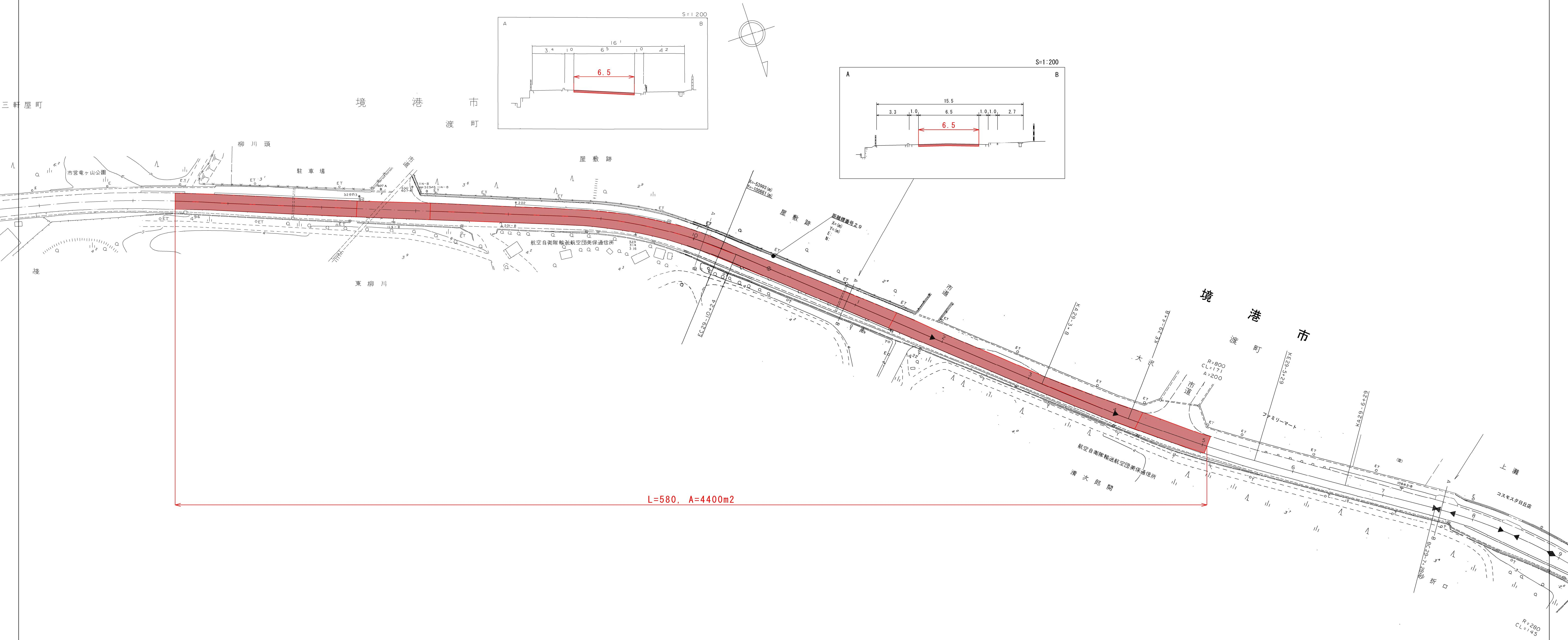
**路面切削工** (t=10cm) A=4400m<sup>2</sup>
